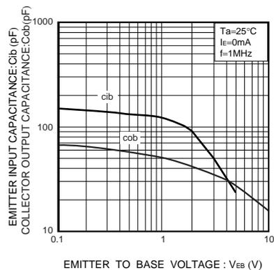
Fig.7 Collector output capacitance vs. collector-base voltage
