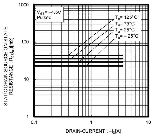
Fig.7 Static Drain-Source On-State Resistance vs. Drain Current(I<sub>D</sub>)
