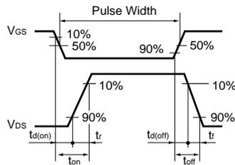
Fig.3-2 Switching Waveforms
