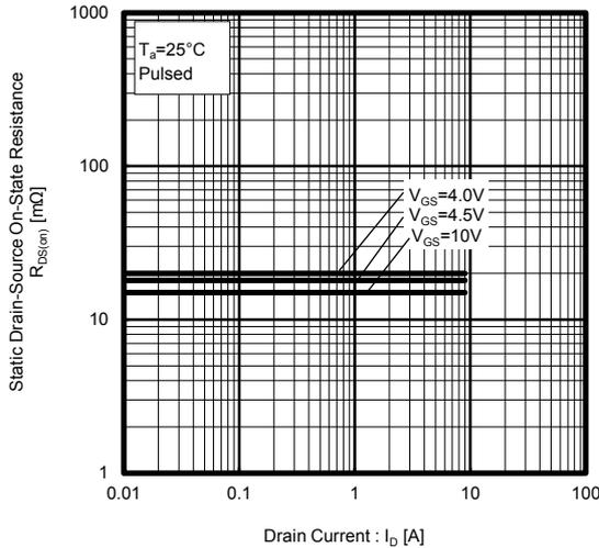
Fig.4 Static Drain-Source On-State Resistance vs. Drain Current
