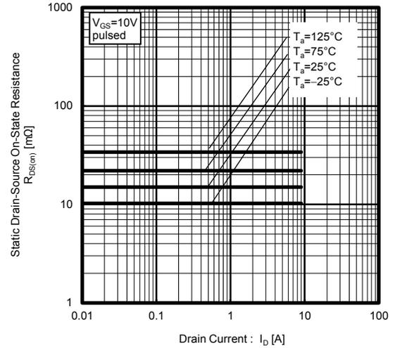
Fig.5 Static Drain-Source On-State Resistance vs. Drain Current
