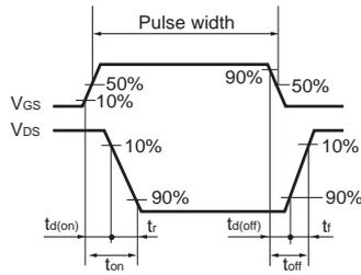
Fig.1-2 Switching Waveforms
