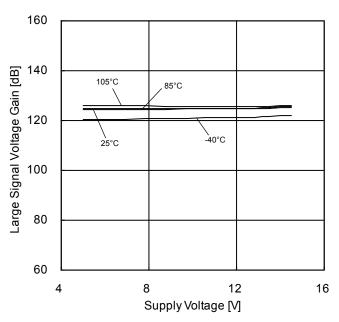
Figure 17. Large Signal Voltage Gain vs Supply Voltage
