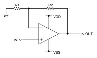
Figure 54. Non-inverting Amplifier Circuit
