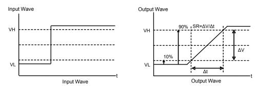
Figure 50. Slew Rate Input Output Wave
