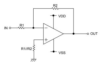
Figure 53. Inverting Amplifier Circuit
