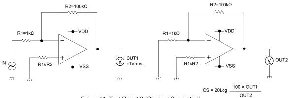
Figure 51. Test Circuit 3 (Channel Separation)
