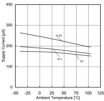
Figure 27. Supply Current vs Supply Voltage
