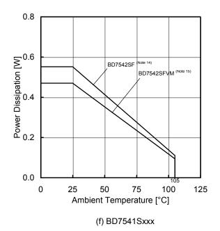
Figure 55. Thermal Resistance and Derating Curve
