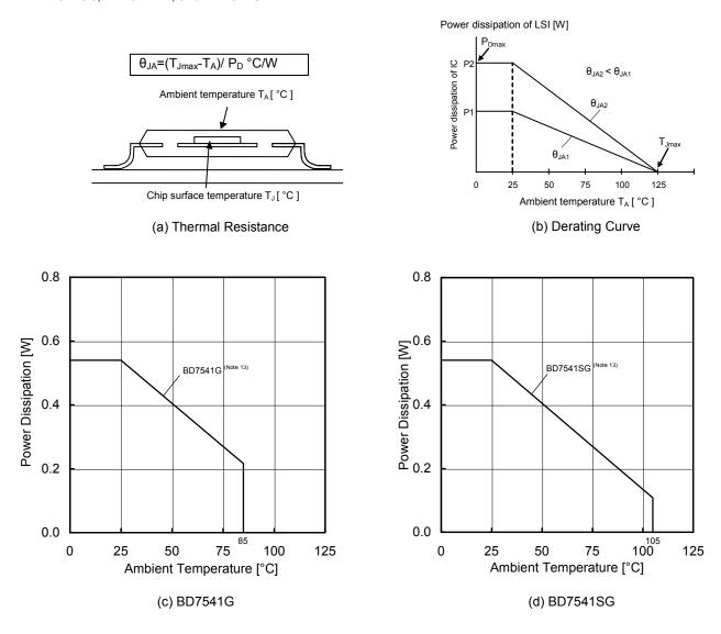
Figure 55. Thermal Resistance and Derating Curve
