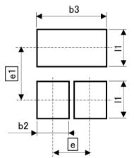
Patterm of terminal position areas [Not a recommended pattern of soldering pads]
