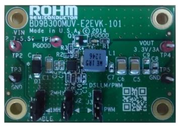
Fig 1: Evaluation Board for the BD9B300MUV
