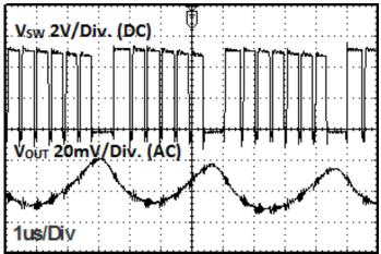
Fig 17: Output Voltage Ripple Response Characteristics (V<sub>IN</sub>=5V, V<sub>OUT</sub>=3.3V, I<sub>OUT</sub>=3A, FREQ=L, MODE=H)
