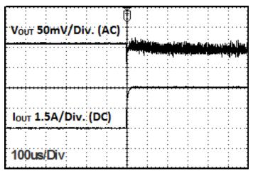
Fig 14: Load Response Characteristics (V<sub>IN</sub>=5V, V<sub>OUT</sub>=3.3V, I<sub>OUT</sub>=0 → 3A, FREQ=L, MODE=H)
