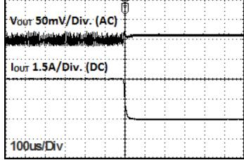
Fig 28: Load Response Characteristics (V<sub>IN</sub>=5V, V<sub>OUT</sub>=3.3V, I<sub>OUT</sub>=0 → 3A, FREQ=H, MODE=H)
