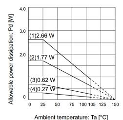
Fig 33: Thermal Derating Characteristics
