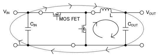
Fig 32: Current Loops of Buck Regulator System
