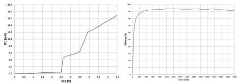
Fig 12: Circuit Current vs. Power Supply Fig 13: Electric Power Conversion Rate Voltage (Temp=25°C, FREQ=L, MODE=H)
