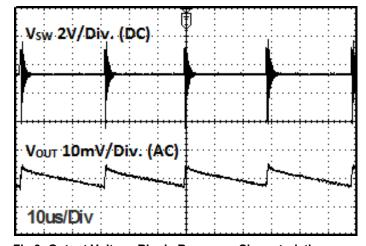
Fig 9: Output Voltage Ripple Response Characteristics (V<sub>IN</sub>=5V, V<sub>OUT</sub>=3.3V, I<sub>OUT</sub>=0, FREQ=L, MODE=L)
