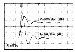
Fig 11: Hot Plug-in Test with Zener Diode P4SMA6.8A, V<sub>IN</sub>=5.5V, V<sub>OUT</sub>=3.3V, I<sub>OUT</sub>=3A, FREQ=L, MODE=H
