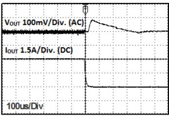
Fig 8: Load Response Characteristics  $(V_{IN}=5V, V_{OUT}=3.3V, I_{OUT}=3A \rightarrow 0, FREQ=L, MODE=L)$
