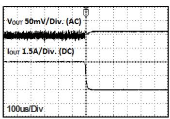
Fig 15: Load Response Characteristics ( $V_{IN}$ =5V,  $V_{OUT}$ =3.3V,  $I_{OUT}$ =3A  $\rightarrow$  0, FREQ=L, MODE=H)
