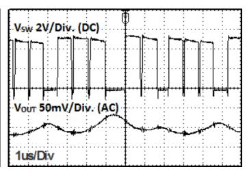
Fig 24: Output Voltage Ripple Response Characteristics (V<sub>IN</sub>=5V, V<sub>OUT</sub>=3.3V, I<sub>OUT</sub>=3A, FREQ=H, MODE=L)
