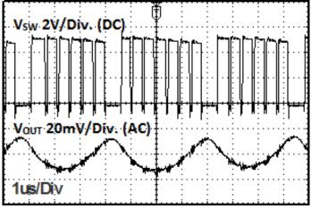
Fig 10: Output Voltage Ripple Response Characteristics (V<sub>IN</sub>=5V, V<sub>OUT</sub>=3.3V, I<sub>OUT</sub>=3A, FREQ=L, MODE=L)
