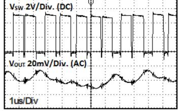
Fig 30: Output Voltage Ripple Response Characteristics (V<sub>IN</sub>=5V, V<sub>OUT</sub>=3.3V, I<sub>OUT</sub>=0, FREQ=H, MODE=H)
